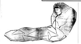
Cosalt thermal protective aid is like an oversized sleeping bag made of plastic. They cam be put on in the water and have a zip up front and hood. They compress down to a small packet that can be stored in the back pouch of your PFD
