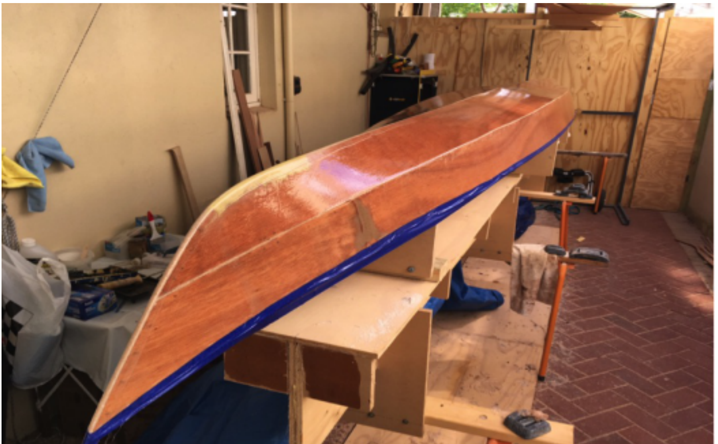
The hull and deck both internally and externally are covered in fiberglass.
