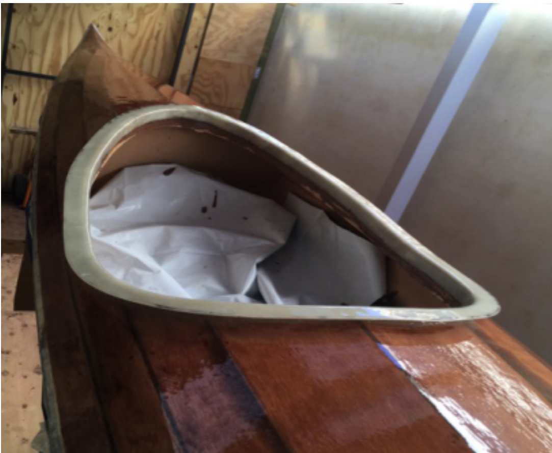
You also make the cockpit rim and hatch recesses out of fiberglass or carbon fibre.
