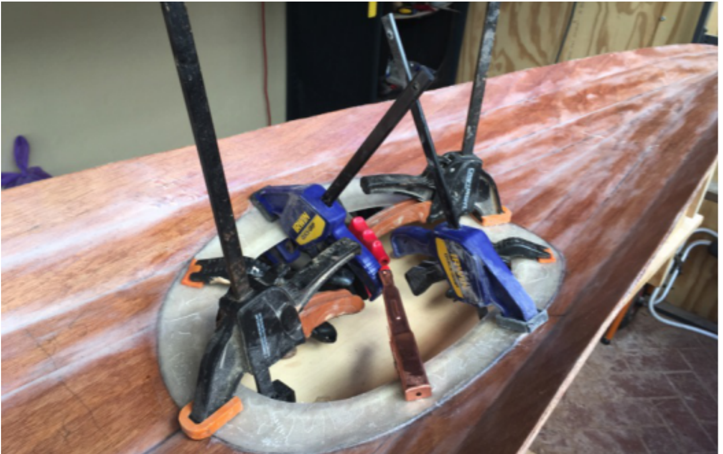
Gluing the hatch recesses to the underside of the deck.
