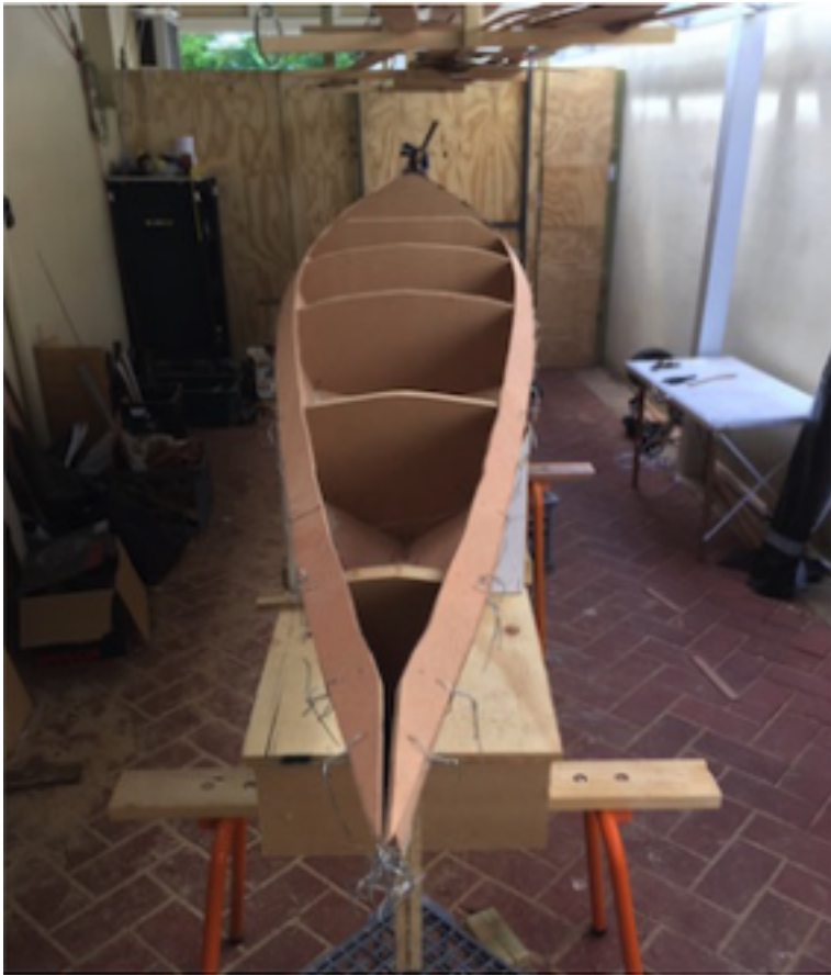
The hull and deck are stitched together before gluing with an epoxy putty.
