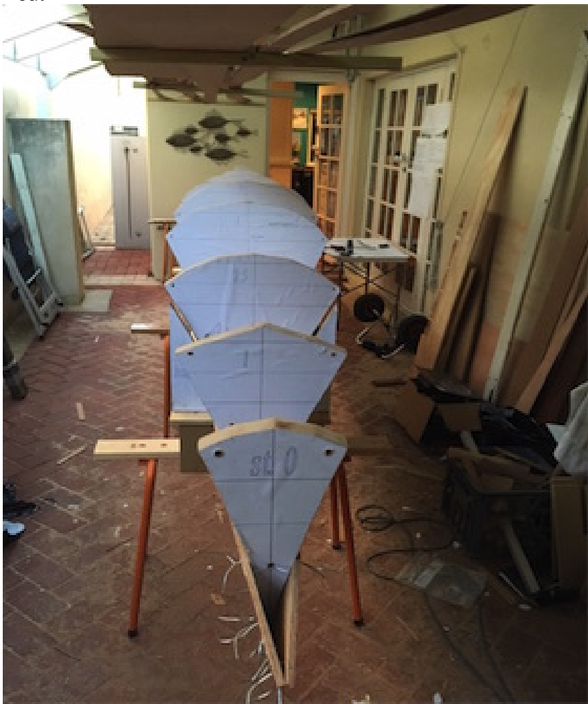
Internal frames are used plus external ones so that the kayak shape is accurate.
